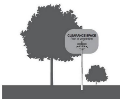
FIGURE 5 – UNINSULATED 66 000 VOLTAGE ELECTRICAL LINE IN A LOW BUSHFIRE RISK AREA AND UNINSULATED ELECTRIC LINE IN A HAZARDOUS BUSHFIRE RISK AREA
