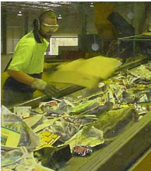
Recyclable material is sorted by a combination of machine and hand sorting. Because of potential danger to workers, plastic bags are not opened. Anything in plastic bags is considered contamination and ends up at landfill.
